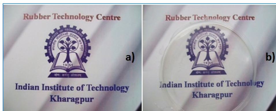
Figure 7. (a) Visibility without block copolymer film. (b) Visibility through transparent PMMA- b -PEHA- b -PMMA triblock copolymer film.
